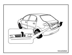
To open the liftgate from outside of the vehicle, insert the key into the lock cylinder and turn it clockwise. Then pull up the handle above the license plate to open the liftgate.
